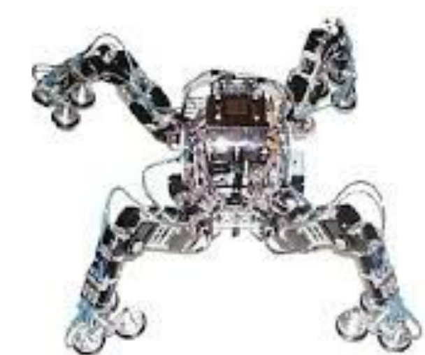
Climbing Robot (Narrow clearance between obstacles)
